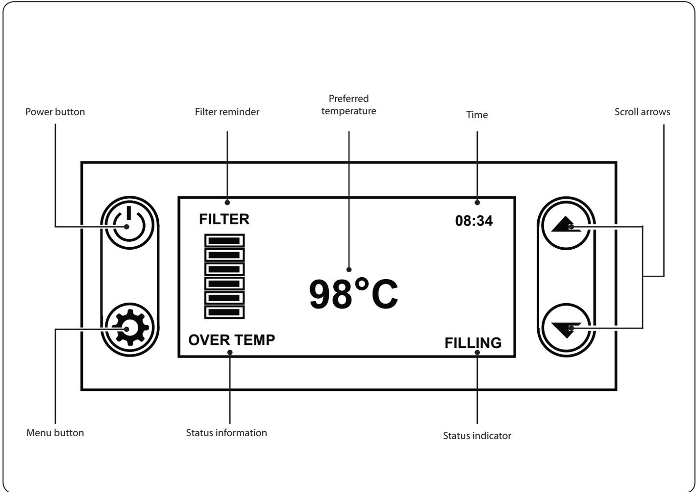
The product has a simple 4 button interface. The display will indicate the status of the boiler and the estimated remaining filter life so you know when to replace the filter. The display has a clear film cover which must be removed.
