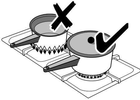
**If a burner flame goes out, turn off the control knob and leave it for one minute before relighting it.**
