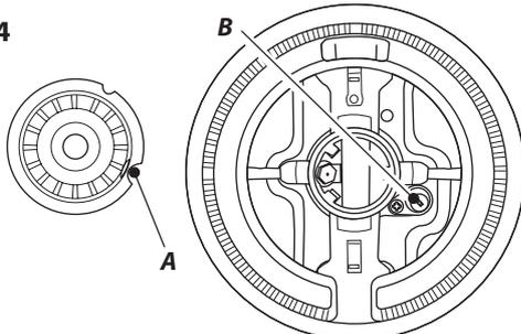
A – Electrode notch, B – Ignition electrode
