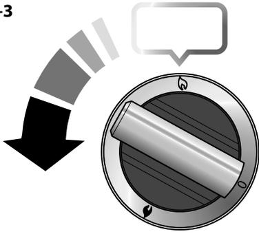
If, when you let go of the control knob, the burner goes out, then the FSD has not been bypassed. Turn the control knob to the OFF position and wait for one minute before you try again, this time making sure to hold in the control knob for slightly longer.
