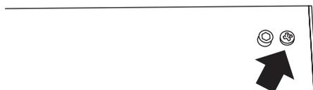
Remove the 2 cross-headed screws that were hidden by the handrail end brackets.
