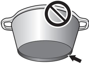
Simmering aids, such as asbestos or mesh mats, are NOT recommended (**Fig. 2.6**). They will reduce burner performance and could damage the pan supports.
