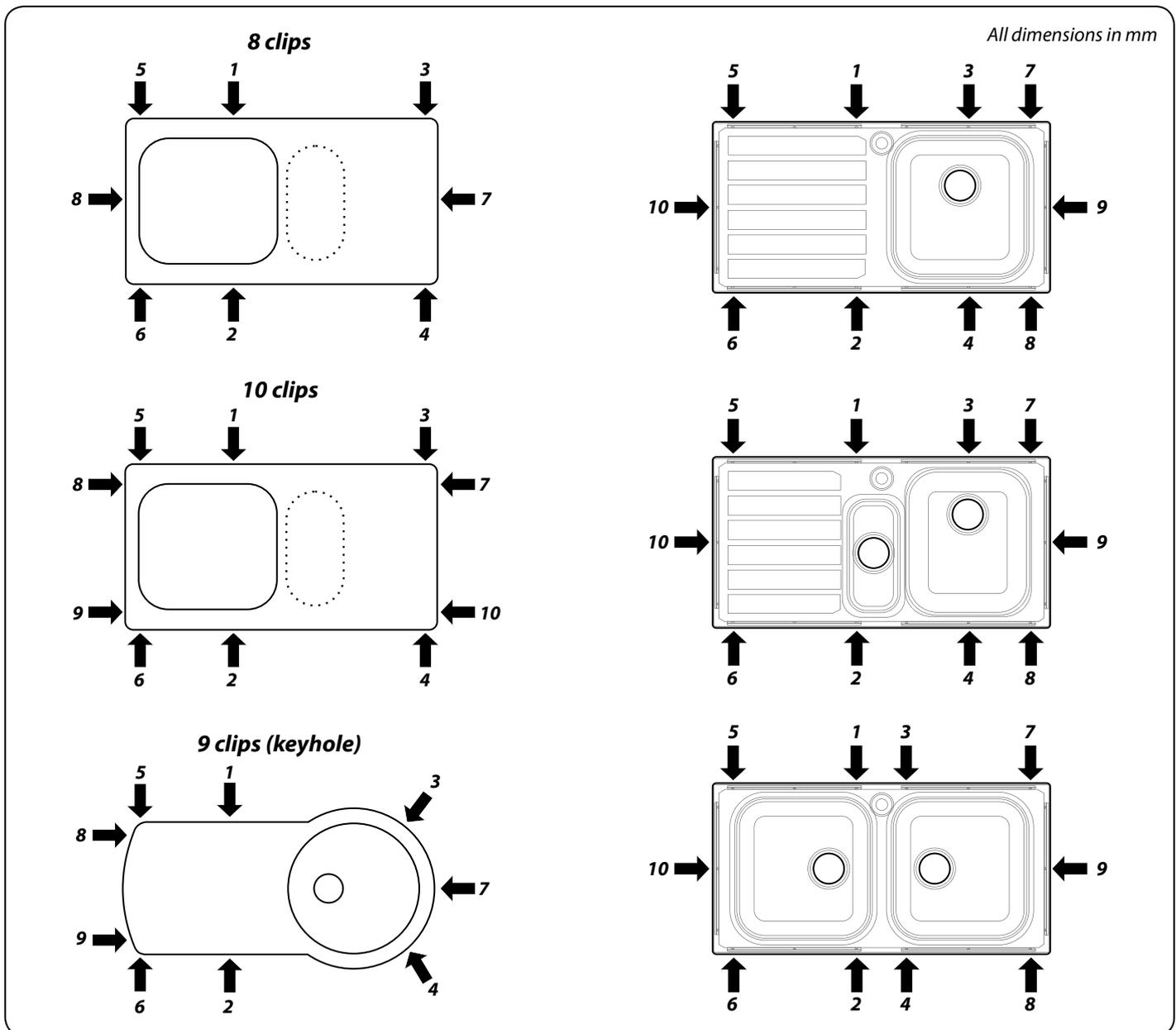
Table 1 Clip positions and recommended tightening sequence
